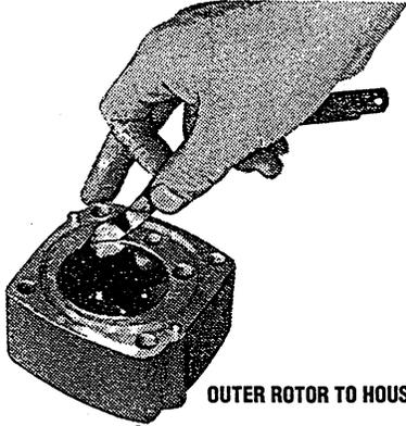
2. **Rotor clearance.** Check the clearance between the outer and inner rotors with a feeler gauge. If excessive, replace the rotor assembly.
