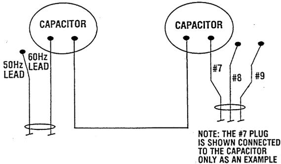
**CAUTION:** Make sure the insulating covers on the unused leads are in place and that the leads never come in contact with each other or come in contact with the case.
