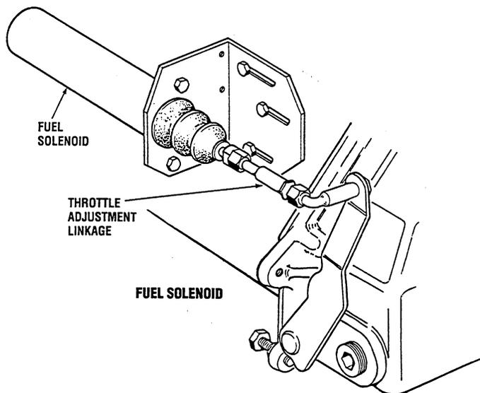
**CAUTION:** Failure of the solenoid plunger to bottom in the solenoid will result in a failed solenoid.
