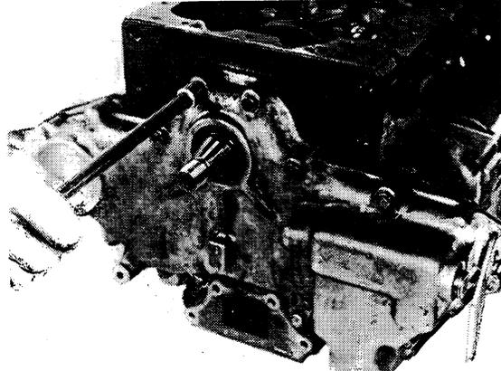
INSTALLING GEAR CASE
