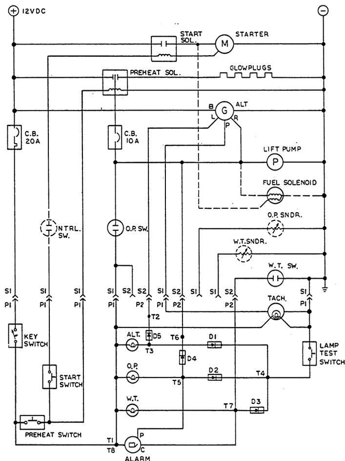
**START:** 1. TURN KEY TO ON POSITION. THE ALARM WILL SOUND, OIL PRESSURE AND BATTERY CHARGE INDICATORS WILL LIGHT.
