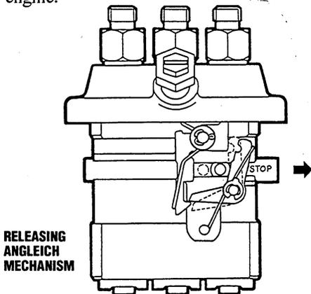
**The inter-cylinder injection control.** Fuel injection control among the cylinders is performed by the adjusting plates (one plate for A Models, two plates for B Models) which have their own cam mechanisms. These adjusting plates are located on the opposite side of the control rack. Necessary turning of the plunger barrels required for inter-cylinder injection control is attained by turning the respective adjusting plates. This adjustment is performed on a fuel shop flow bench only.
