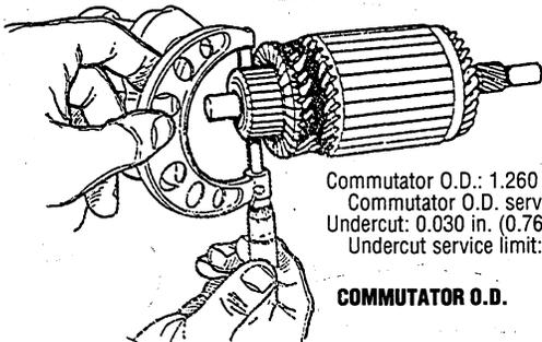
Commutator O.D.: 1.260 in. (32.0 mm)
