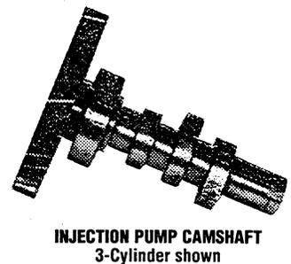
**The high-pressure oil pump** is directly coupled to the injection pump camshaft at the rear of the shaft, mating into the Oldham's coupling groove.
