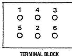
Residual voltage measured between line to neutral will be 4–6 volts AC between each pair of leads at the terminal block. This would be an indication that the stator windings are OK. Check exciter windings and artificially excite the generator.
