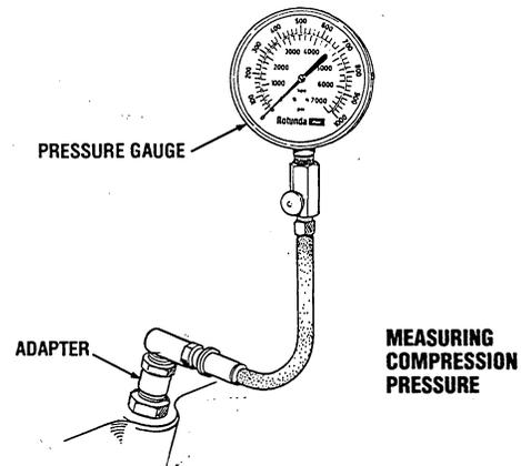
7. Crank the engine with the starter motor until the pressure reaches a maximum value. Read the engine rpm and the pressure gauge when the starter rotation has become stable.
