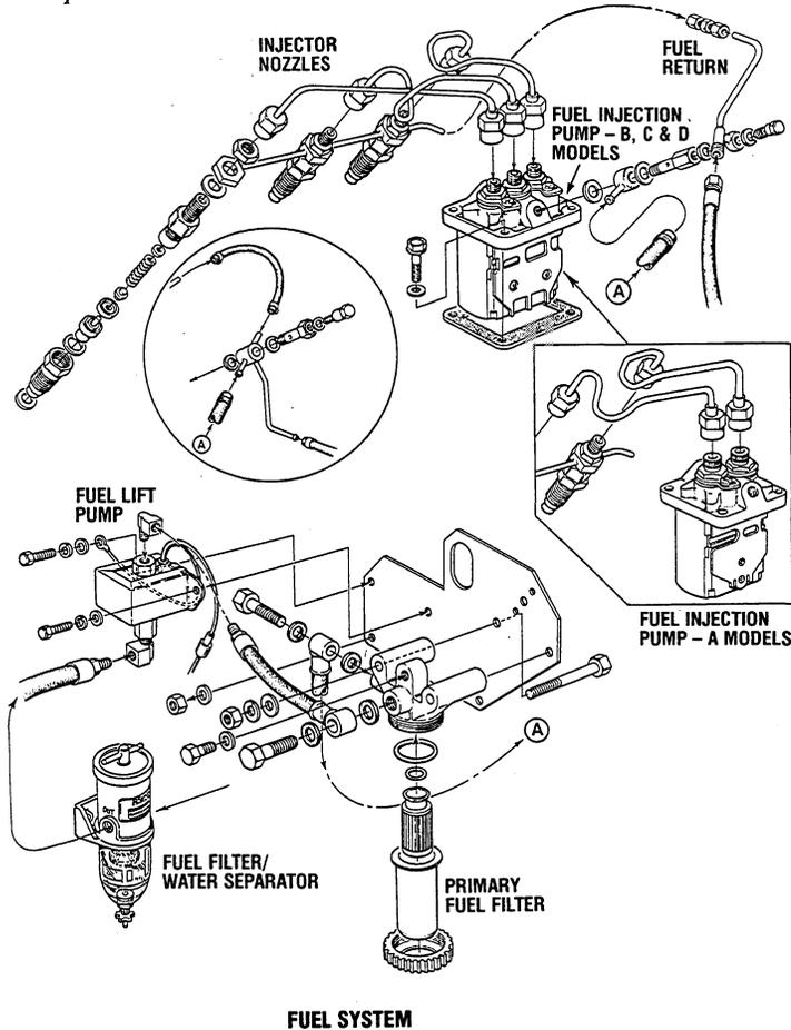
The **built-in fuel injection pump** is mounted on the right side of the cylinder block. It consists of the pump elements (plunger assemblies), delivery valves, tappets and smoke set unit. As the pump camshaft rotates, the plungers are moved up and down through a fixed stroke, thus delivering pressurized fuel to engine cylinders.
