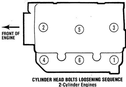
CYLINDER HEAD BOLTS LOOSENING SEQUENCE
