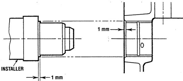
PRESS-FITTING CAMSHAFT BUSHING
