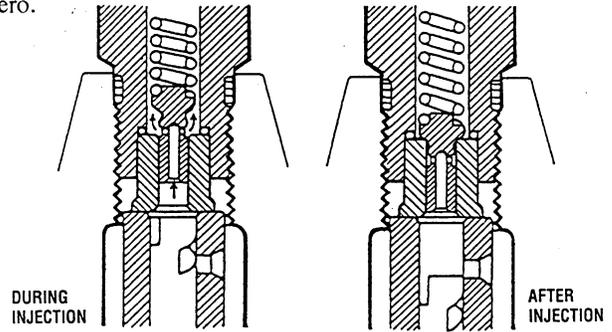
**Nozzle and nozzle holder.** Fuel from the fuel injection pump flows through the passage in the body of each nozzle holder and is injected from the nozzle into the combustion chamber. Fuel overflowing from the nozzle enters the nozzle holder and returns to the fuel tank through the banjo and attached return fuel line.
