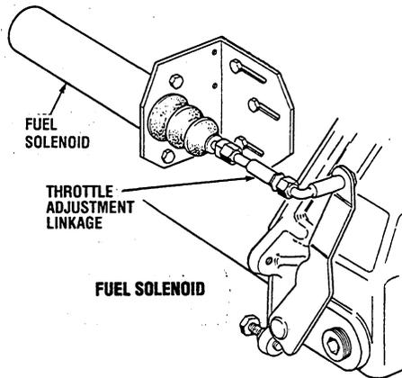
**CAUTION:** Failure of the solenoid plunger to bottom in the solenoid will result in a failed solenoid.
