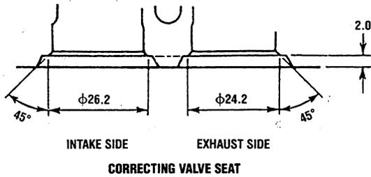
2. If the valve seat sinkage reaches the replacement value (see *SERVICE STANDARDS*), install a new valve seat.
