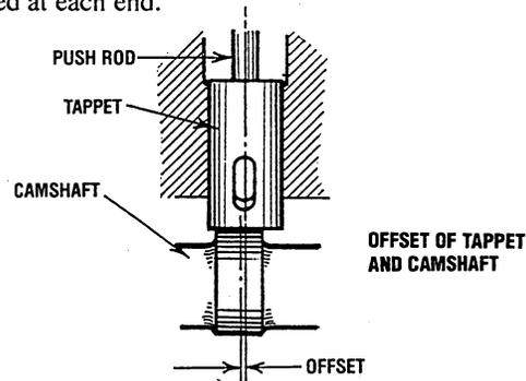
**The injection pump camshaft** is made of high carbon steel. Its cam surfaces are induction-hardened to improve wear resistance. The front end of the shaft supported on a ball bearing is connected to a gear. The rear end is provided with an Oldham's coupling groove for connecting to the oil pump drive shaft.
