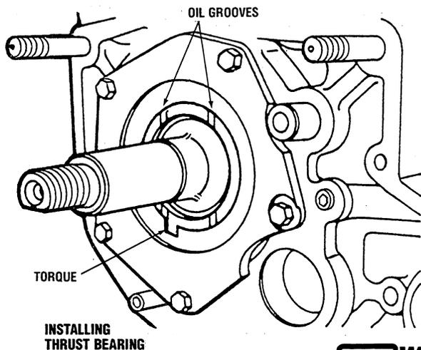
5. Install the outside thrust bearing in the bearing bore in the bearing housing, then install the stopper plate, crankshaft gear and sleeve. Install the stopper plate with the chamfered side facing toward the rear of the engine. Install the crankshaft gear with the stepped side facing toward the rear of the engine. Also install the sleeve with the chamfered square end toward the front of the engine.
