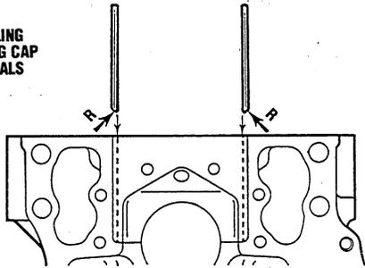
9. Install the oil seal into the crankshaft rear oil seal case. Install the seal case to the cylinder block. Remember to install the gasket. Turn the crankshaft one complete revolution to ensure there is no unwanted binding.
