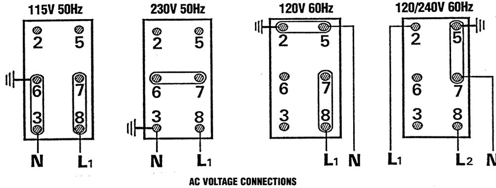
**NOTE:** The frame ground wire must be moved when changing from 120 volts and 120/240 volts 60 hertz to 220 volts 50 hertz. For making connections to the AC terminal block, use terminal ends for 1/4" studs that will accept multi-strand copper wire sized for the amperage rating from the hot lead connection.
