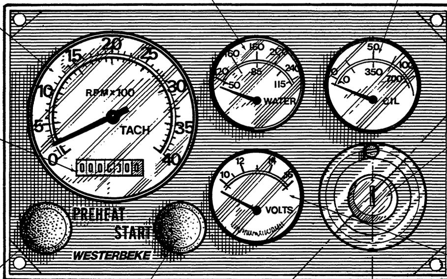
**PREHEAT BUTTON:** WHEN PRESSED, ENERGIZES THE ALTERNATOR'S REGULATOR, THE FUEL LIFT PUMP AND THE ENGINE'S GLOW PLUGS. IT BY-PASSES THE ENGINE'S PROTECTIVE OIL PRESSURE ALARM SWITCH. IN ADDITION, THIS BUTTON ENERGIZES THE START BUTTON.
