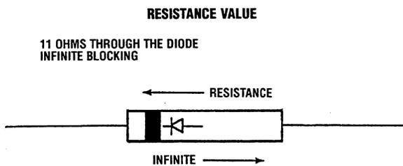
The diodes can be easily checked in place with the use of a common automotive 12-volt high beam headlight bulb, some jumper leads, and the generator's 12 volt starting battery (see the next page).
