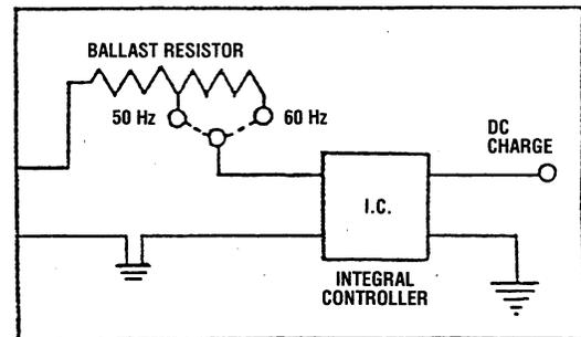
Early controllers having this resistor in the DC charging circuit are of the three-lead type. These three-lead types consist of either three spade plugs in connections, or three wire leads coming from the controller.
