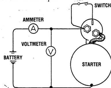
**CAUTION:** Use thick wires as much as possible and tighten every terminal securely. This is a solenoid shift-type starter which makes a rotating sound louder than that of a direct-drive type starter. When detecting starter rotation at the pinion tip, be careful not to come in contact with the pinion gear when it protrudes.
