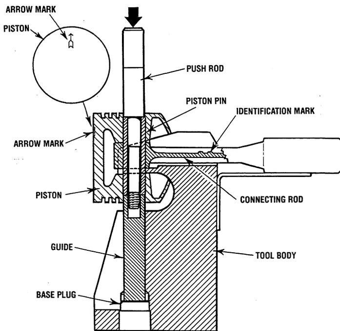
INSTALLING PISTON PIN
