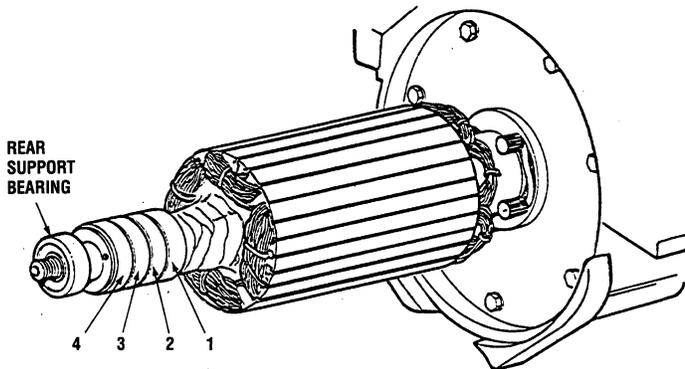
3. For a residual voltage check, disconnect the field leads from the bridge rectifier. Note the position of the leads on the rectifier (+) to (+) and (-) to (-). Operate the generator and check the AC output (no load on generator). Measure the voltage between the neutral lead and the hot lead(s) (3 and 4 wire unit — 2.5 volts AC each hot lead to neutral approximate).
