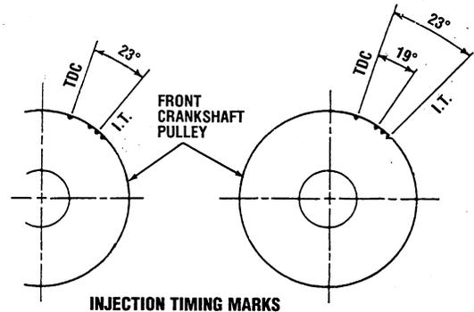
8. When the specified injection timing is not correct, increase or decrease the shim material thickness under the fuel injection pump's mounting flange. Injection timing varies 1° with each 0.1 mm increase or decrease of shim thickness. The addition of shim thickness will retard the timing and reducing shim thickness will advance the timing. Shims are available in the following thicknesses: .2 mm, .3 mm, .4 mm and .8 mm. Refer to your engine's/generator's parts catalog for shim part numbers.
