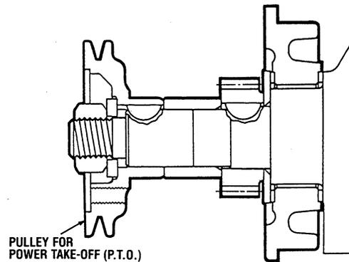
6. Temporarily install the sleeve stopper, washer (except for the P.T.O. pulley) and crankshaft pulley. Tighten the nut. Check the crankshaft end play. If the end play exceeds the specified value, recheck the thrust bearing. Also check that the crankshaft gear and sleeve are properly installed. After checking the end play, loosen the nut and remove the pulley and washer.
