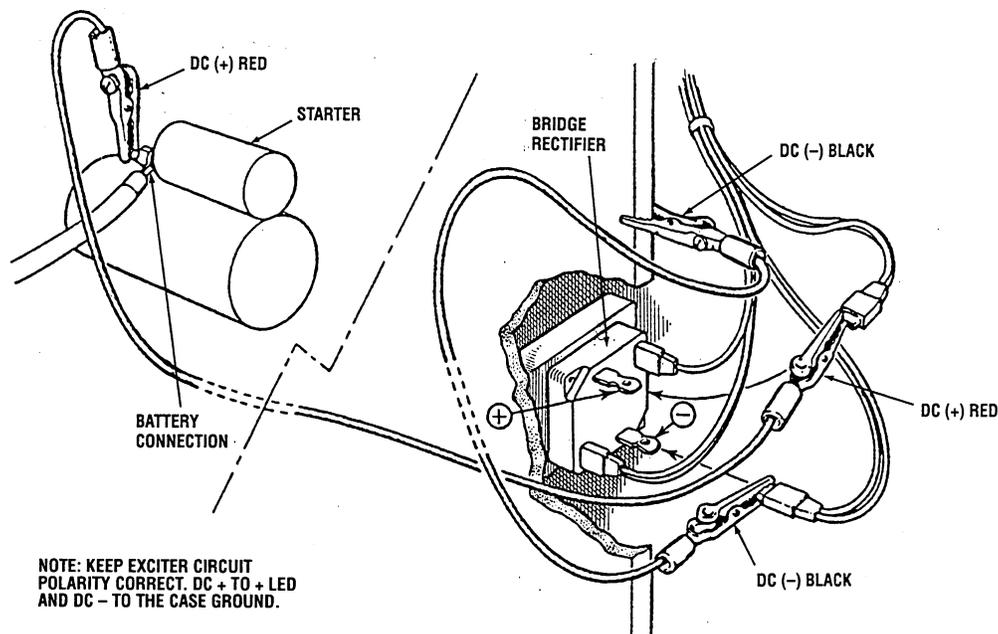
NOTE: KEEP EXCITER CIRCUIT POLARITY CORRECT. DC + TO + LED AND DC - TO THE CASE GROUND.
