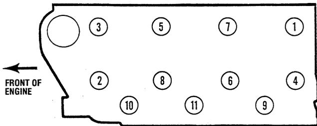
CYLINDER HEAD BOLTS LOOSENING SEQUENCE
